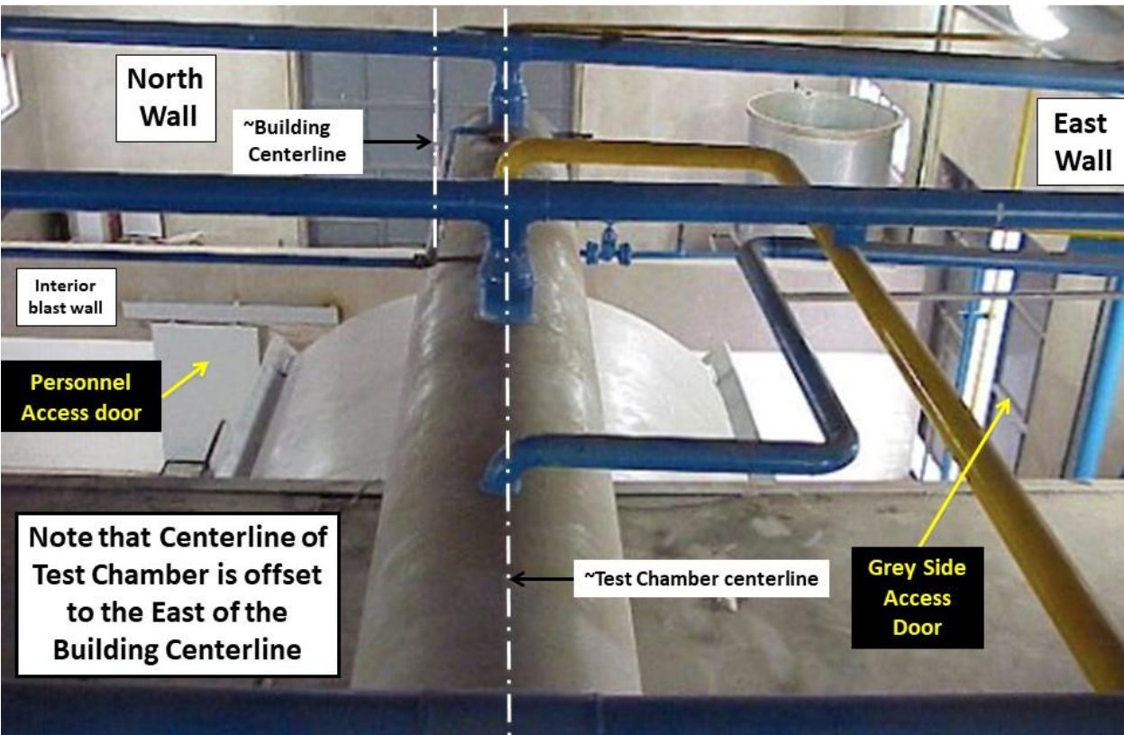
Figure 7. Image from the archive seized by Israel and made available to the public. As discussed in the text, it shows a high explosive test chamber at the Parchin site. Annotations by the Institute.
