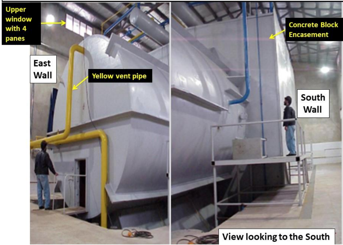
Figure 4. Image from the archive seized by Israel and made available to the public. As discussed in the text, it shows a high explosive test chamber at the Parchin site. Annotations by the Institute.
