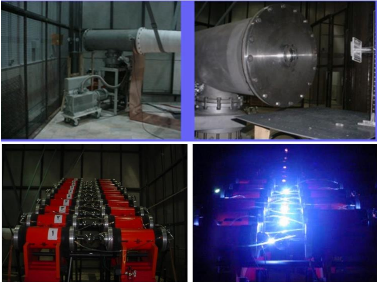
Figure 15. Flash X-Ray system for nuclear-related testing in Taleghan 2 (upper). Below is a Marx generator in Taleghan 2 used as part of a flash x-ray to deliver fast pulses of energy to enable a rapid succession of images to be taken.
